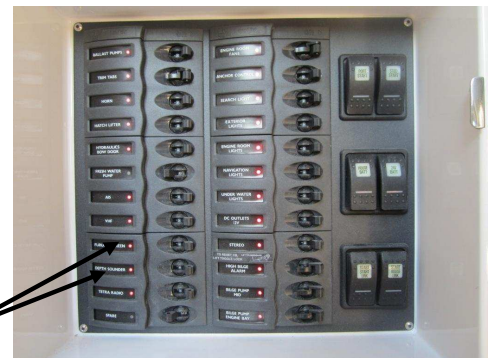
Circuit breakers for the Furuno screen and depth sounder module
