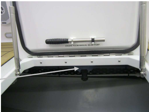
Engine room discharge whale manual bilge pump located in the port tank room hatch
