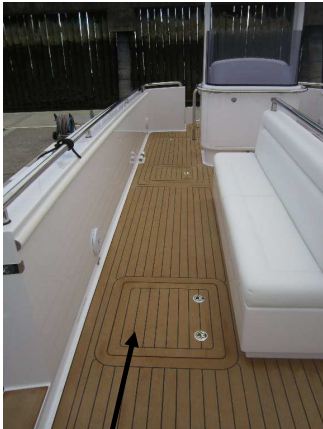
Mastervolt chargers located via starboard tank room hatch
