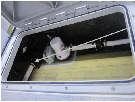
Manual Bilge Pump, pick-up, forward engine room bulkhead
