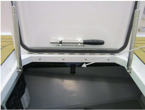
Tank room discharge whale manual Bilge Pump, located in the starboard tank room hatch
